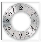
**13 Chapter ring,** silver-coloured, satin-finish aluminium with printed numerals. Outside Ø 182.5 mm, inside Ø 102 mm, 0.4 mm thick. For hand lengths 75–88 mm.
