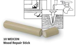
Two-component plasticine for fast, permanent repair of wooden parts. For repairing cracks, drill holes, broken out and broken off wooden parts and seals joints. Temperature resistant from -35 to +120 °C. Can be mechanically machined and painted. Adheres to wood, metal, ceramics, glass, many plastics. Content 56 g.
