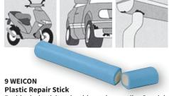
Residual elasticity, durable and versatile. Specially for repairs on plastic parts and fibre composite materials as well as metal, wood, glass and ceramic parts. Easily portionable, temperature resistant from -50 to +120°C, processing time 20 min., curing time 3 hrs, final strength after 36 hrs. Cures virtually shrink-free, can be mechanically processed and over painted. Content 57 g.
