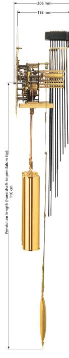
**7-day rope movement** with change-over strike train. 3 classic chimes – 4/4 Westminster, St. Michael and Whittington – can be set manually or can be selected automatically to sound a different chime every 3 hours. Precision clock with tray escapement, automatic anchor, bronze bushings and seconds display. Power reserve during winding. Automatic overnight silencing (10.15 p.m. to 7 a.m.) or complete switching off of the hour and / or quarter strike can be selected.
