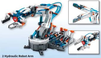
The hydraulic robot arm is simply controlled by water pressure - without a motor, without a battery. In this case the robot is extremely flexible, the gripper can be activated so that objects can be raised and lowered. The robot is composed of 229 components and is constructed with the aid of illustrations, recommended for 10 years and above.
