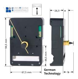
**Equipment:** Case with integrated antenna. Fully automatic time setting and changing (3 to 10 minutes) with 2 motors. Complete with 80-mm second hand and installation kit (see INFO below). Without hanger (order no. 242399, p. 9) Please order pair of hands separately!
