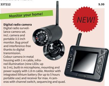
With stand and power supply. Recording of video and sound at the press of a button onto SDHC card (card not included). Dimensions: Ø 42 x 92 mm (camera), 130 x 90 x 27 mm (monitor).
